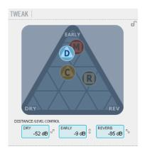
The relation between the Dry, Early and Reverb levels defines the perceived distance of a source. The less dry signal compared to Early and Reverb levels, the greater the perceived distance. Early and Reverb levels set the relation between the amount of room definition compared to the reverb diffuse field.
