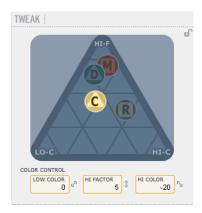
The Color parameter controls are advanced controls handling the sonic specter of the Reverb diffuse field. Try adding a bit of HiColor if you feel the level of reverb is correct but still doesn't stand out as you intended.
