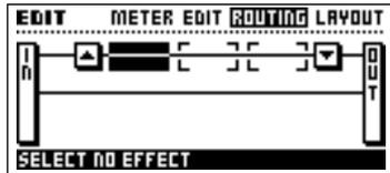
The difference between the three modes is, that the processing sample rate in the first mode is 44.1 or 48 kHz, where it is 88.2 or 96 kHz in the other two modes. The arrow boxes on each side of the processing blocks indicates the up and down sampling of the signal.
