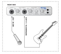
Konnekt 24D can be used with no computer connected as a stand-alone unit still providing both the excellent mic pre-amps and Hi-Z inputs on channels 1 and 2. It is even possible to use the included Fabrik R (reverb) and Fabrik C (channel strip & comp).
