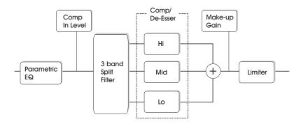
This is a schematic overview of the signals flow through the algorithm in 3-band mode. As illustrated - the signal first passes the 4 band parametric EQ. Then the signal is split into Io-, mid- and hi-bands for individual compression. Cross-over frequencies between the bands are set by the selected Source type.
