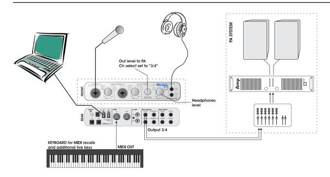
This example illustrates how Konnekt integrates perfectly in a live setup. The objects in a live setup could be:
